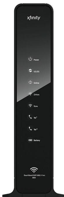
The integrated router features a Dynamic Host Configuration Protocol (DHCP) server, Network Address Translation (NAT), Network Address Port Translation (NAPT), and a stateful packet inspection (SPI) firewall. These features allow the user to share a single high-speed public Internet connection and to share files and folders between devices in the home network by attaching multiple wired and wireless devices in the active home or office to the wireless residential gateway.
