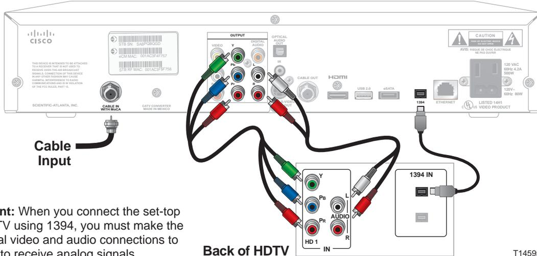
**Important:** When you connect the set-top to your TV using 1394, you must make the additional video and audio connections to your TV to receive analog signals.
