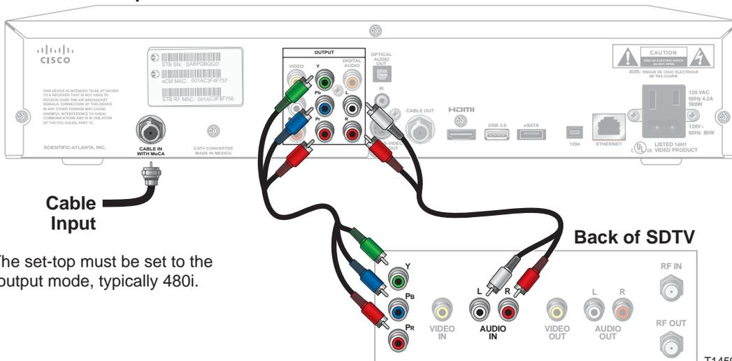
**Note:** The set-top must be set to the proper output mode, typically 480i.
