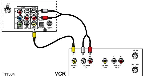
The program that you are copying appears in the *PIP window*. Connecting to your VCR using the **OUT 2** outputs allows you to watch or record another program or even change channels in the Main screen, without affecting the copy in progress.
