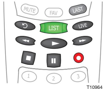
While in normal play mode, press **Rewind** or **Fast-Forward** to cycle through three different speeds of rewind or fast-forward.
