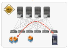
L2 & L3 Wire-rate Overlay / Underlay VXLAN / BGP Control Plane Third Party Controllers
