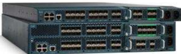
Figure 2. Cisco UCS 6120XP 20-Port Fabric Interconnect (Top) and Cisco UCS 6140XP 40-Port Fabric Interconnect
