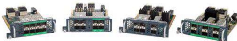
Figure 6. From left to right: 8-Port 1/2/4-Gbps Native Fibre Channel Expansion Module; 4-Port Fibre Channel plus 4-Port 10
