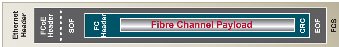
Figure 3. In FCoE, the Fibre Channel payload is encapsulated in Ethernet frames.
