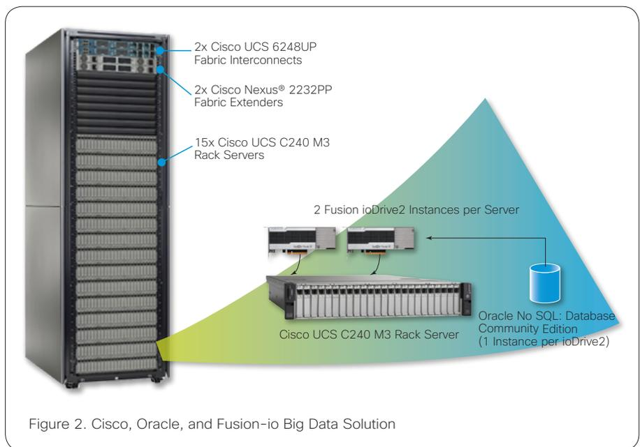
Figure 2. Cisco, Oracle, and Fusion-io Big Data Solution
