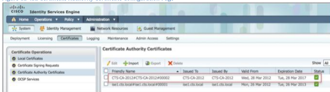
Figure 12 ISE Certificate Authority Certificate Configuration Page
