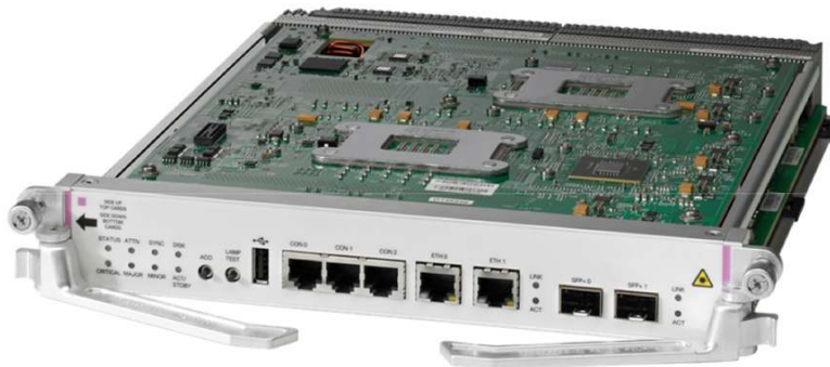
Figure 4. Route Processor Line Card
