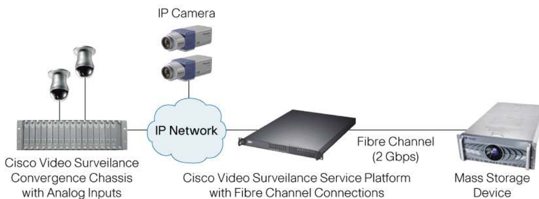
Figure 2. Cisco Video Surveillance Services Platform with Fibre Channel Connections in a Video Surveillance Deployment
