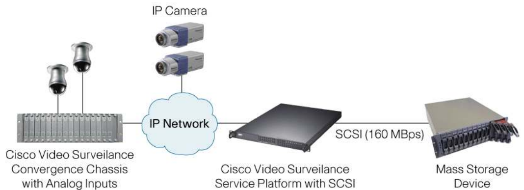
Figure 2. Cisco Video Surveillance Services Platform with SCSI in a Video Surveillance Deployment
