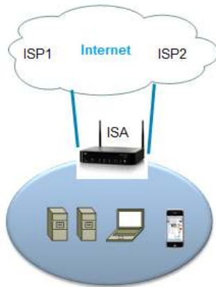
Figure 3. Cisco ISA500 Use Case: VPN Gateway at Multiple Company Locations
