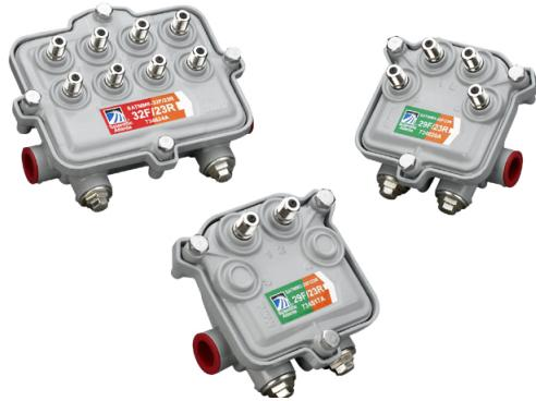
In the forward path, the tap loss in the Reverse Window tap is deliberately down-tilted, with greater loss at higher frequencies than at lower frequencies. This enables more frequent use of high value taps - increasing system design efficiency, and improves the ability to optimize tap port levels.
