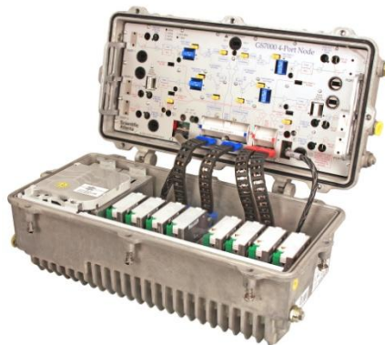
Figure 1. GS7000 4-Way Segmentable Node with 65/86 MHz Split
