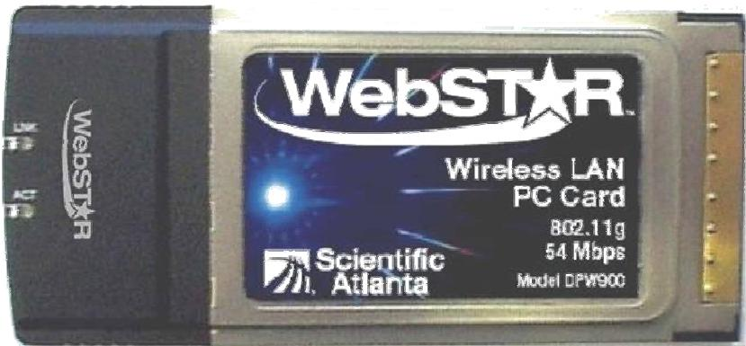
The DPW900 is designed and built to meet the 802.11g wireless specifications and offers data rates up to 54 Mbps. It is also backward compatible with 802.11b networks. In addition to providing the data connection to the PC from the wireless network, the PC Card interface also provides power to the wireless adapter and eliminates the need for an external power supply.
