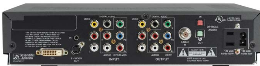
3250HD rear panel showing optional loop-through connections
