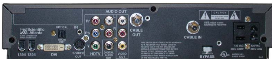
3250HD rear panel showing optional IEEE 1394 digital outputs
