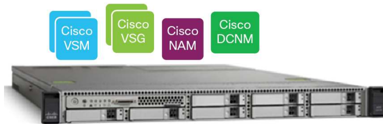
Figure 2. Cisco Nexus 1100 Series with Four VSBs: Cisco VSMs, VSGs, NAM, and DCNM
