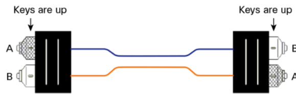
Figure 7. Type A-to-B Jumper Fiber Mapping (per TIA-568-C.3)
