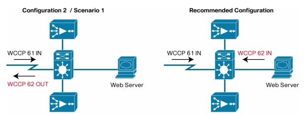
Figure 6. Configuration 2/Scenario 1 Network Diagram Comparison to Recommended Configuration
