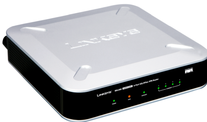
Figura 1. Router SSL/IPsec VPN de 4 puertos Cisco RVL200
