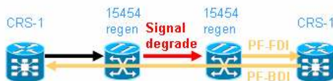
Figure 13. Proactive Fast Reroute Feature Avoids Traffic Slowdowns
