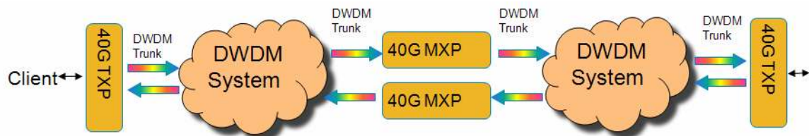
Figure 6. Unidirectional Configuration for 40-Gbps Muxponder in Regeneration Mode
