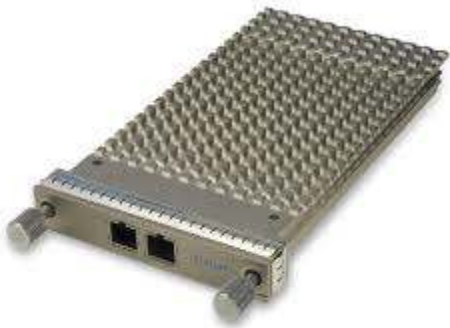
Figure 9. A CFP Transceiver Module from the Cisco ONS family
