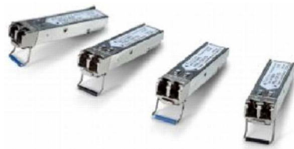
Figure 7. An SFP+ Transceiver Module from the Cisco ONS family
