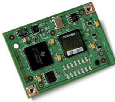
Figure 2. Cisco 2-Port T1/E1 MFT VWIC2 with 64-Channel MFT Dedicated ECAN Module
