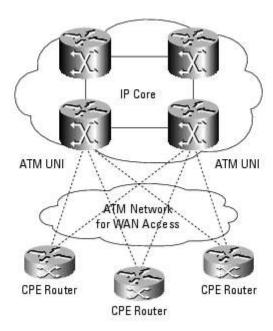
Using the Cisco 7600 Series ATM line cards, service providers can interconnect their points of presence (POPs) via a core ATM network. (See Figure 3.)
