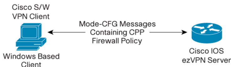
Figure 110. EasyVPN Dynamic Firewall/Access Control List Policy Push to Cisco VPN Software Client
