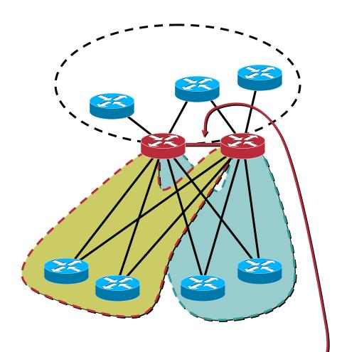
Trunk with One VLAN in Each Flooding Domain
