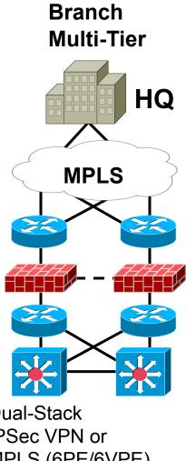
**Dual-Stack** IPSec VPN or MPLS (6PE/6VPE) Firewall (IPv4/IPv6) Switches (MLD-snooping)
