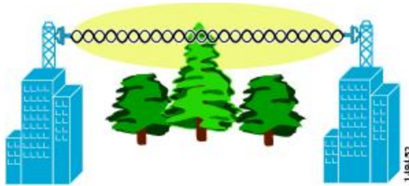
Figure 25: Typical Obstructions in a Fresnel Zone
