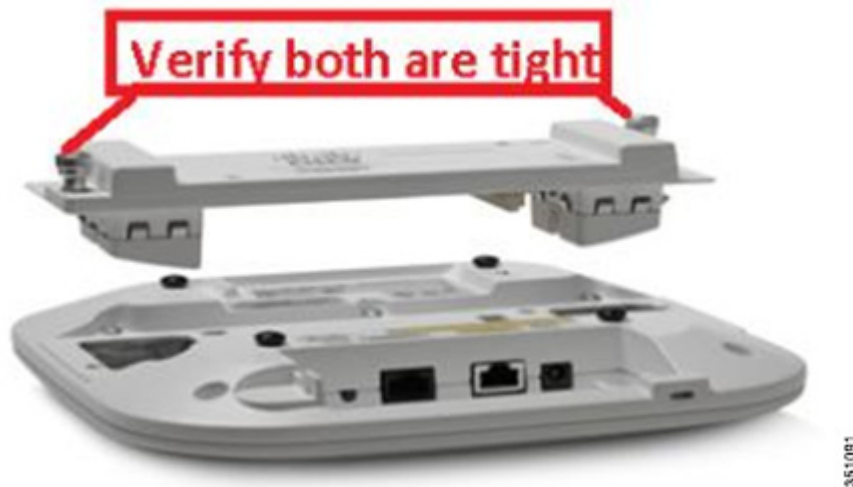
Figure 74 Both thumbscrews need to be tight or power is not applied
