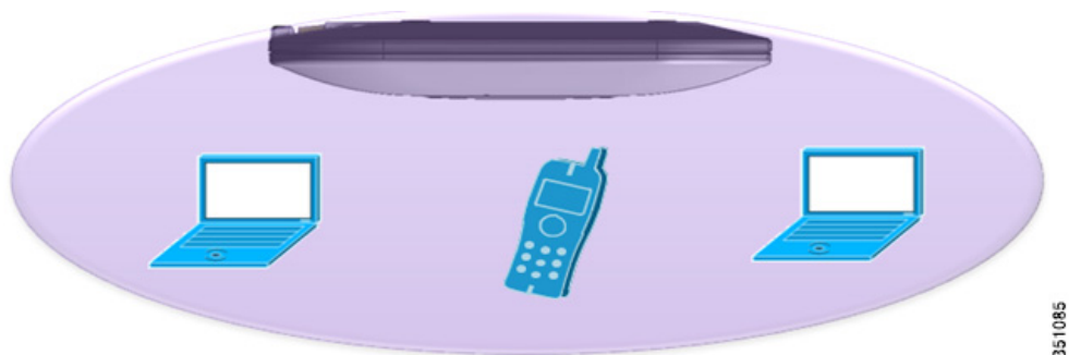
Figure 68 Coverage is optimized for ceiling placement and radiates omni-directionally
