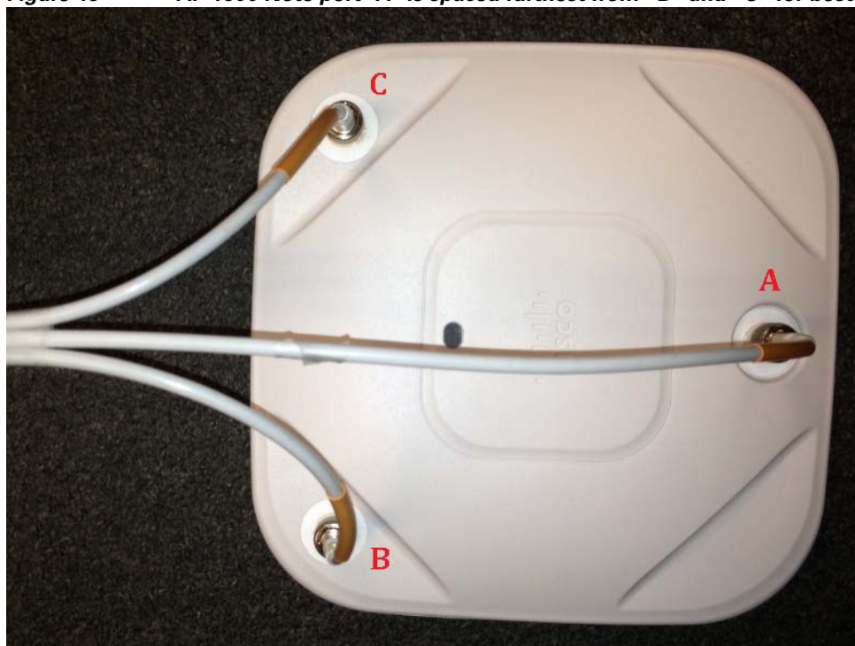
Figure 46 AP 1600 Note port “A” is spaced furthest from “B” and “C” for best diversity
