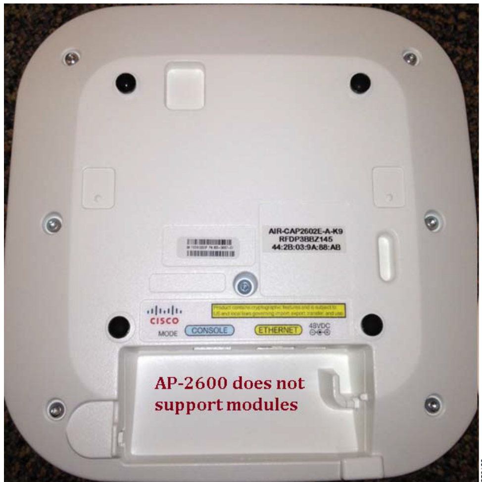
Figure 10 Backside of the AP 2600 - mounting hardware and antennas are the same as AP 3600
