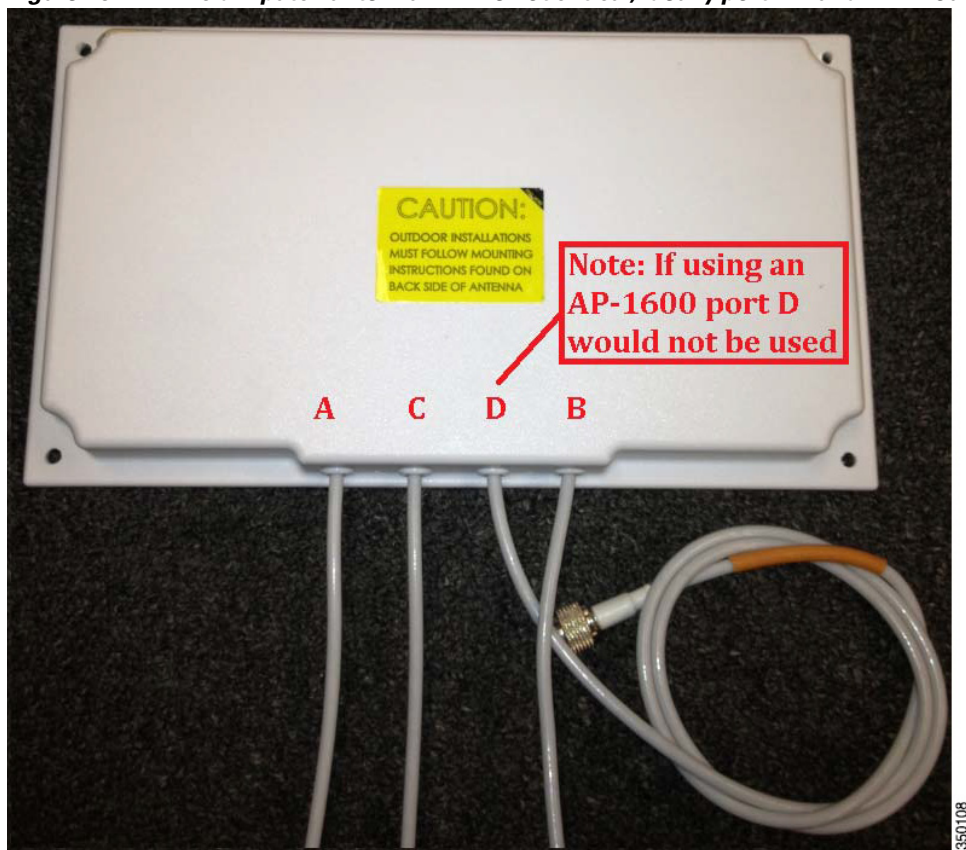
Figure 45 6 dBi patch antenna – while not critical, ideally port “A” and “B” would be on the ends.
