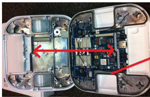
Figure 22 Inside of the AP 3600 - (no vents or fans, everything is industrial quality)
