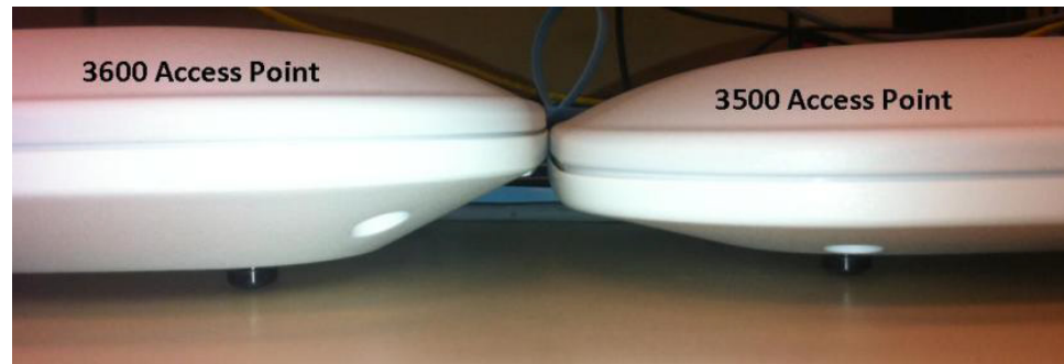
Figure 6 Side View of AP 3600 (2.11 inches) and AP 3500 (1.84 inches) in height
