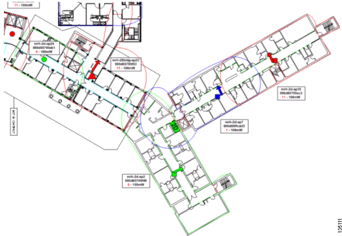
Figure 1-7 Hospital Floor Survey by a Survey Crew
