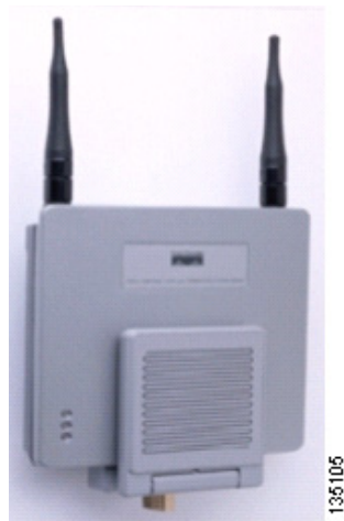
Figure 5-5 Access Point Mounted on a Wall
