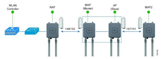
High gain directional antenna should be used in typical serial backhaul deployments. In addition, "Preferred Parent" configurations should be used to create serial backhaul mesh networks.
