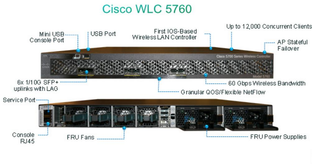
CT5760 controllers will be deployed behind a core switch/router. The core switch/router will be the only gateway into the network for the controller. The uplink ports connected to the core switch will be configured as EtherChannel trunk to ensure port redundancy.
