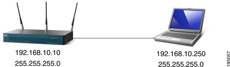
If you use this method, you will need to reconfigure the cabling for subsequent startup and deployment of the access point so that the access point is no longer connected directly to the PC but instead is connected to the LAN (either by using a hub or a switch).
