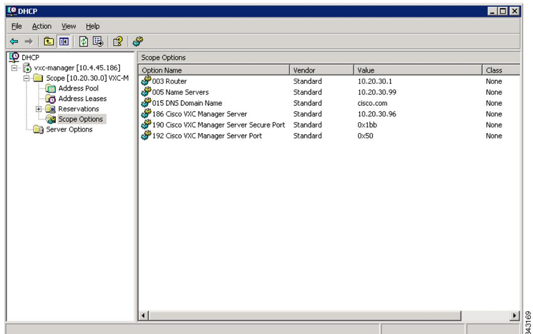
**Step 10** Confirm that options 186, 190 and 192 are listed with proper values under the target DHCP server and scope.
