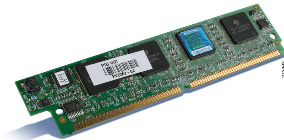
Figure 54 64-Channel Packet Fax/Voice DSP Module
