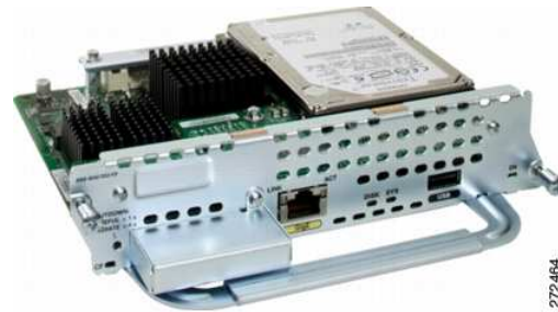
Figure 57 Cisco Unity Express Network Module
