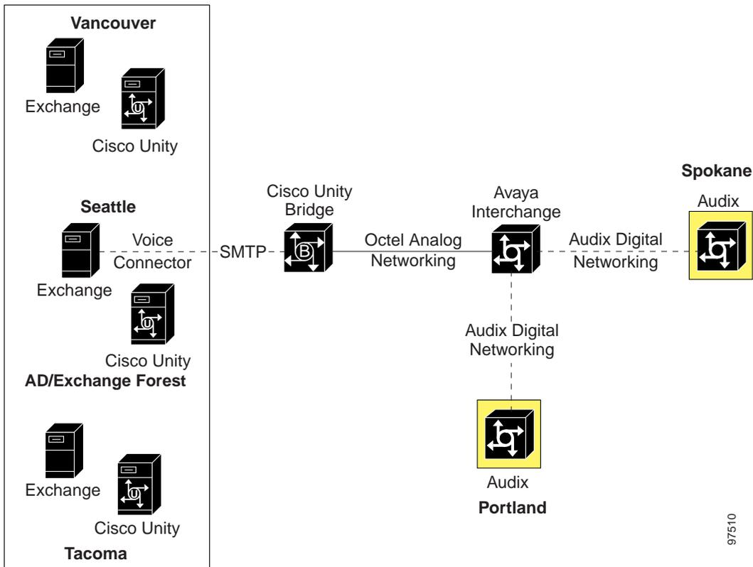
There should be no need to edit the configuration on the remaining Portland and Spokane servers because they are already configured to route messages to Vancouver network addresses through the Interchange.
