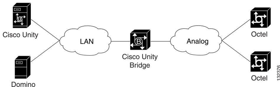
However, as [Figure 1-3](#) illustrates, the Bridge server can be located in a different location from Cisco Unity and Domino, in which case messages are sent through the Internet or a WAN.
