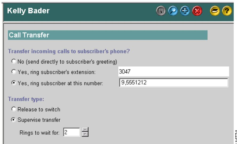
When the call transfer setting is set to “No (send directly to subscriber’s greeting),” the call transfer number is automatically set to the subscriber extension (3047 in the example above), which is replicated to the other networked Cisco Unity servers.
