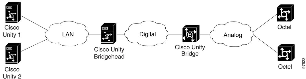
Because the analog transmission of messages to the Octel servers is much slower than digital transmission to Cisco Unity, the bridgehead server can be configured for networking with additional Bridge servers, as needed, to provide sufficient analog ports for messaging with the Octel servers.
