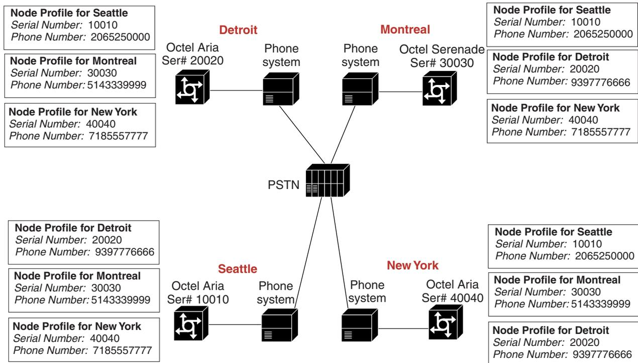
The Bridge and Cisco Unity bridgehead servers can represent one or more nodes in the network. Both the Bridge and Cisco Unity bridgehead servers must be configured with information about the other Octel nodes. The Bridge and Cisco Unity bridgehead servers must also be configured with information that identifies the nodes that they represent.
