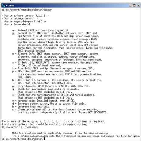
**4** Type **doctor -g** and then press **Enter** to view the version of DNCS software installed and the DNCS and Application Server platform, CPU, and disk information.
