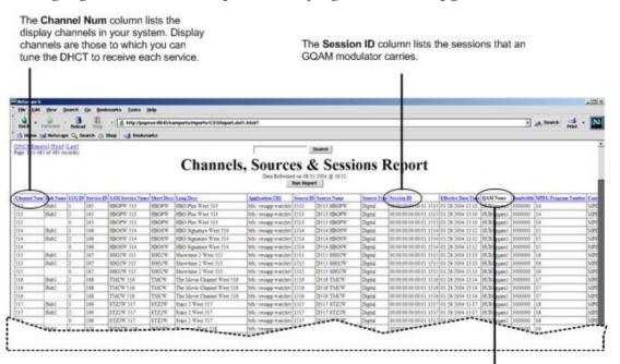
The QAM Name column lists the name of each GQAM modulator, uniquely identifying each GQAM modulator in the system.
