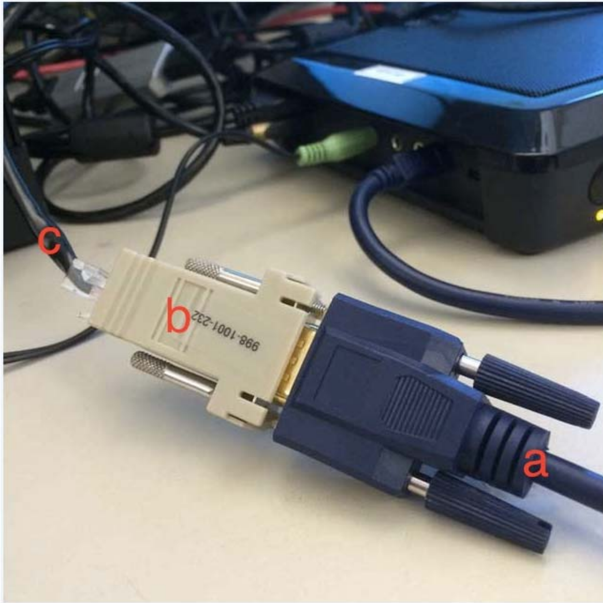
Figure G-3 Cables for RS-232 Control Input
