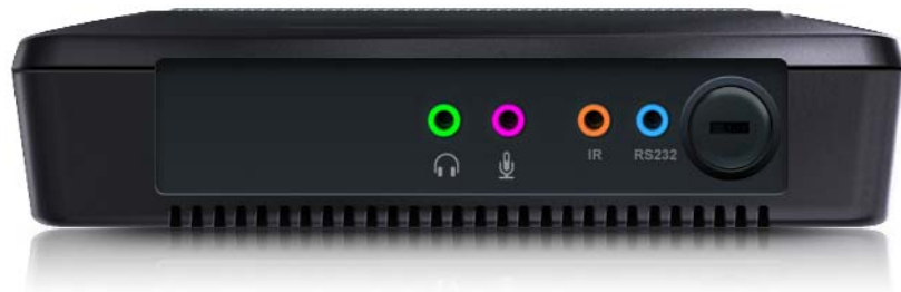
Figure 7-5 The TRS audio connectors on the Cisco IEC 4600 Series
