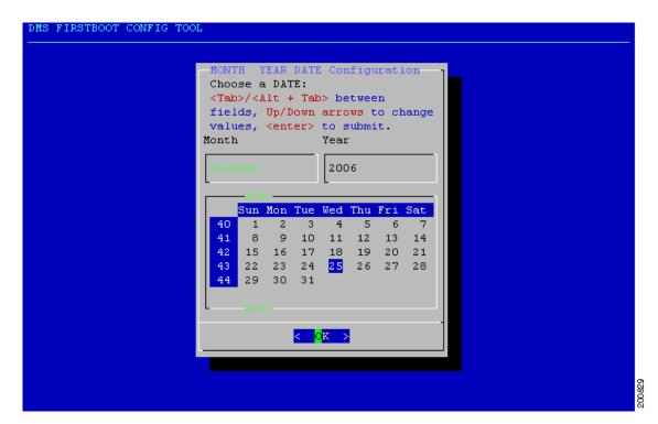
Step 20 Confirm the date. Press Enter if the information is correct. If you need to change the information, use the arrow keys to navigate to No and press Enter to reconfigure your settings.
