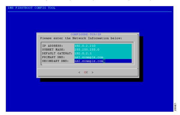
Step 12 Confirm the network settings. The following example reflects the sample configurations specified above. Press Enter if all the information is correct. If the information is incorrect, use the arrow keys to navigate to no and press Enter to re-configure your settings.
