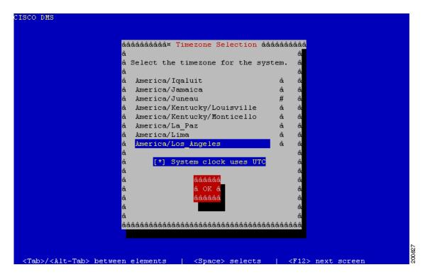
Step 18 Confirm the time zone setting. Press **Enter** if all the information is correct. If any information is incorrect, use the arrow keys to navigate to **No** and press **Enter** to re-configure your settings.
