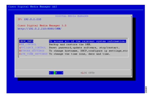
**Step 2** To back up or restore the DMM, select **BACKUP\_DMM** as shown:
