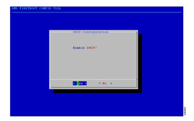
**Step 11** If DHCP is not enabled, enter the IP address, subnet mask, default gateway, primary DNS and, if available, a secondary DNS in the Configure TCPIP screen.
