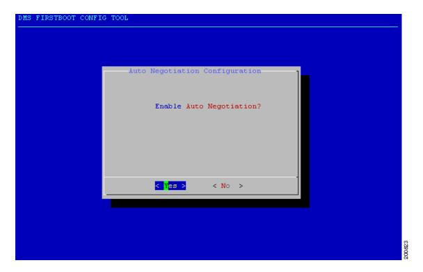
**Step 14** If you turned on autonegotiation, go to time zone configuration (Step 17). If autonegotiation is not turned on, set the NIC speed to 10, 100, or 1000 Megabits.
