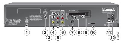
1 Cable In Connects to a coaxial cable that delivers the signal from your service provider
