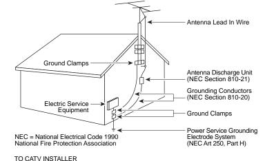
This reminder is provided to call the CATV system installer's attention to Article 820-40 of the National Electrical Code (NEC) that provides guidelines for proper grounding, and in particular, specifies that the cable ground shall be connected to the grounding system of the building, as close to the point of entry as practical.
