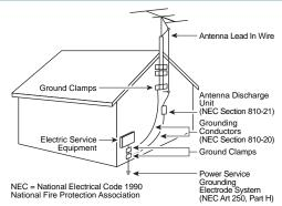
TO CATV INSTALLER This reminder is provided to call the CATV system installer's attention to Article 820-40 of the National Electrical Code (NEC) that provides
