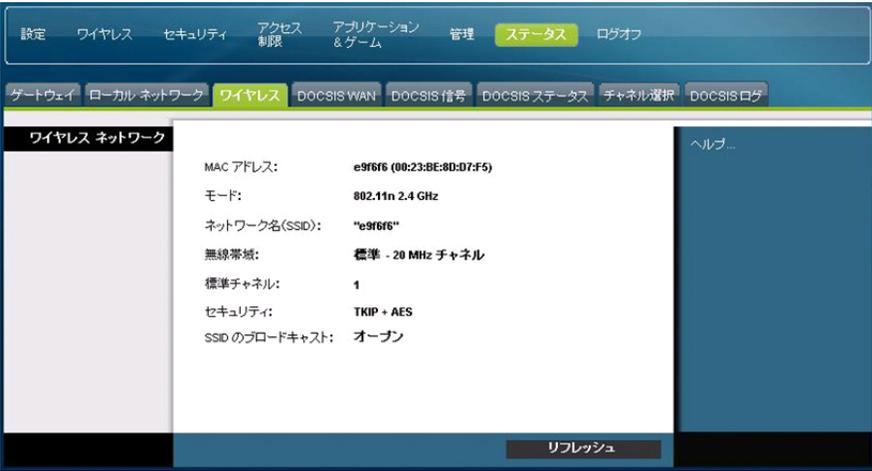
The screenshot shows the 'ワイヤレス ネットワーク' (Wireless Network) status page. It displays various configuration details for the wireless network, including the MAC address, mode, SSID, channel, and security settings. A 'リフレッシュ' (Refresh) button is visible at the bottom.
