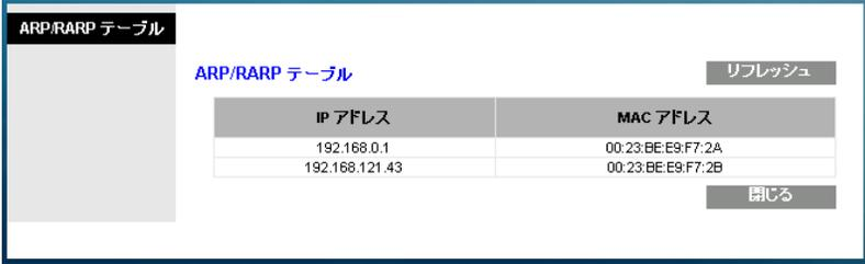
The screenshot shows a web interface for the ARP/RARP table. It features a table with two columns: 'IP アドレス' and 'MAC アドレス'. The table contains two rows of data. Above the table is a 'リフレッシュ' (Refresh) button, and below it is a '閉じる' (Close) button.
