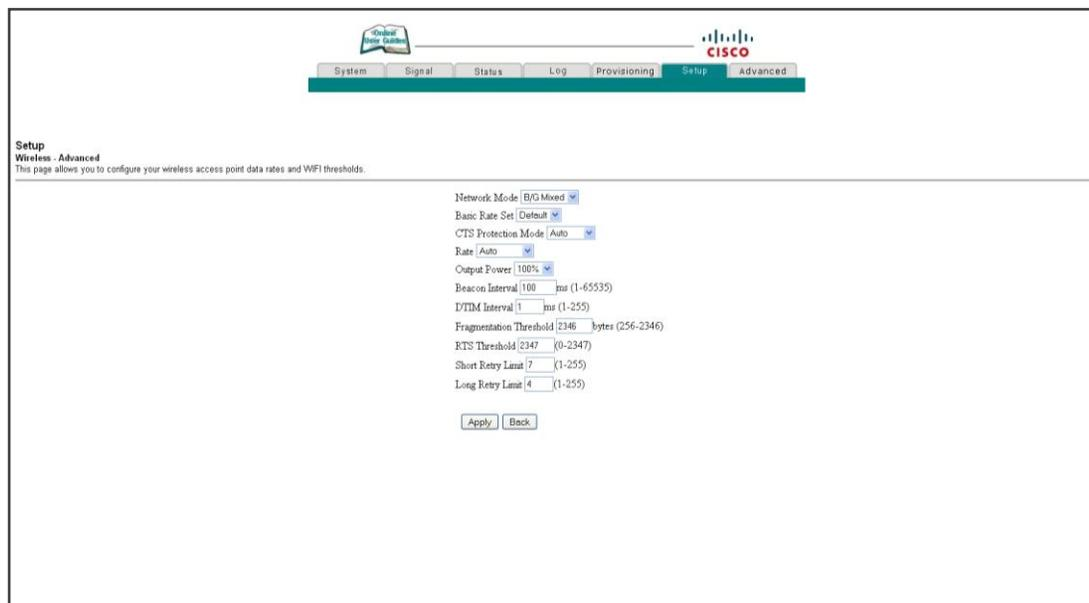
The screenshot shows the Cisco configuration interface for "Setup Wireless - Advanced". The page title is "Setup Wireless - Advanced" and the subtitle is "This page allows you to configure your wireless access point data rates and WFI thresholds". The configuration parameters are as follows:
