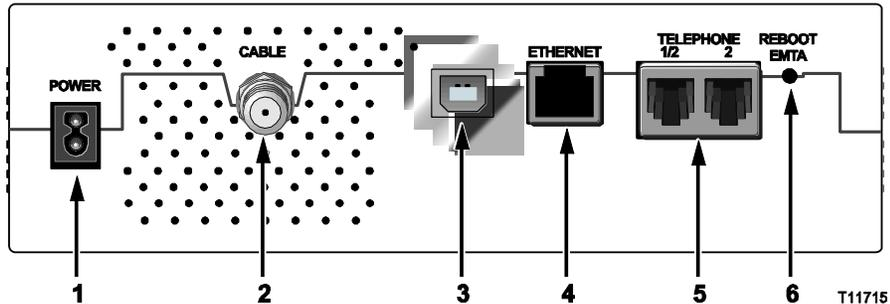
**Important!** Do not connect your PC to *both* the Ethernet and USB ports at the same time. Your modem will not function properly if both the Ethernet and USB ports are connected to your PC at the same time.
